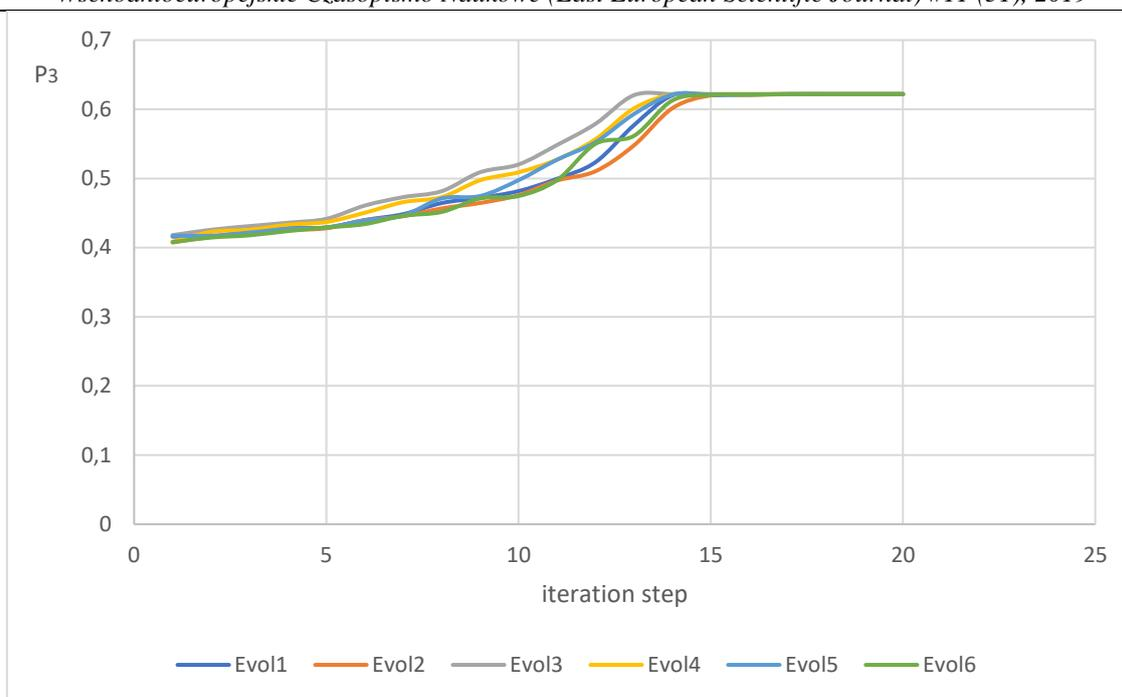
Fig. 5 Graph of the search for points of maximum efficiency of the solar collector, by the method of evolutionary search.
