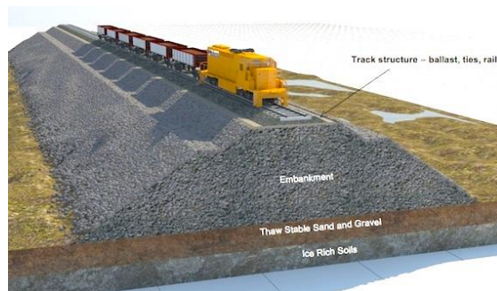
Fig. 7. Sketch of train at the railway embankment
