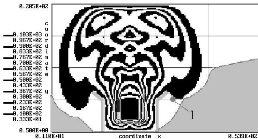
Fig. 5. Dimensionless sound pressure field near railway track, t=0.008s (scenario #3: vertical barriers with wings)
