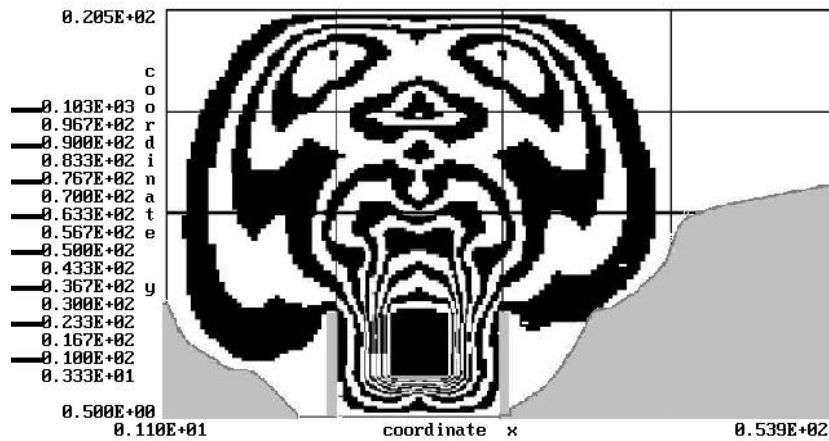
Fig. 4. Dimensionless sound pressure field near railway track, t=0.008s (scenario #2: vertical barriers)
