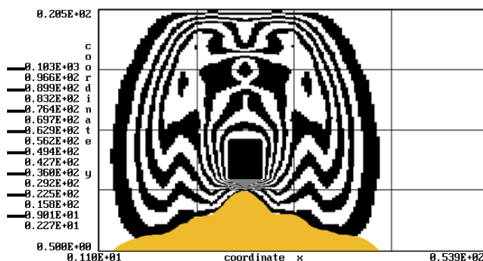
Fig. 8. Dimensionless sound pressure field near railway track (scenario #1: no barriers)
