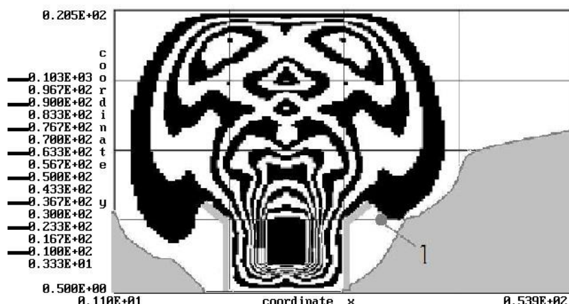
Fig. 5. Dimensionless sound pressure field near railway track, t=0.008s (scenario #3: vertical barriers with wings)
