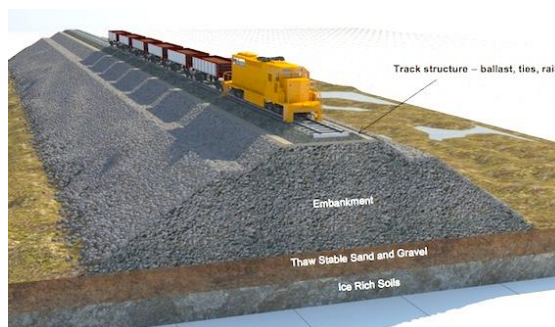
Fig. 7. Sketch of train at the railway embankment
