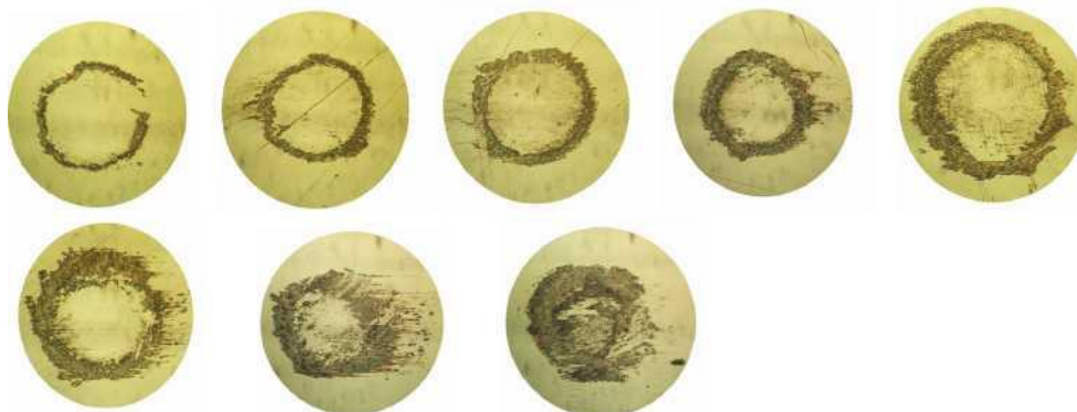
Fig. 3. Evolution of the contact zone of the sample with fluctuations in the scheme of a metal ball (12.7 mm) and a flat surface
