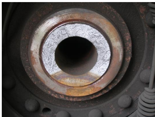
Fig.1. View of the section of the right axle of the front wheels of the car's semitrailer
