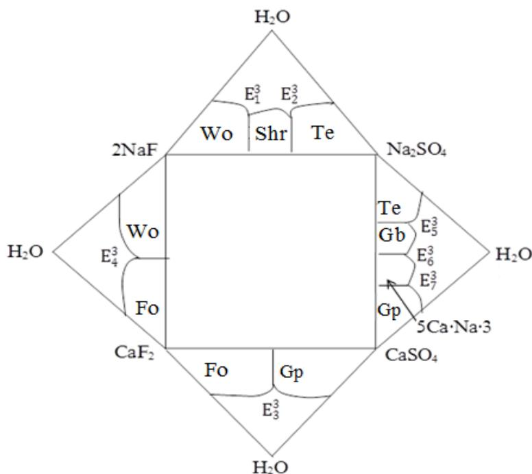
*Figure 1. Phase equilibria diagram of the Na, Ca// SO4, F - H<sub>2</sub>O system at 75°C at the ternary composition shown in the form of an unfolded pyramid.*
