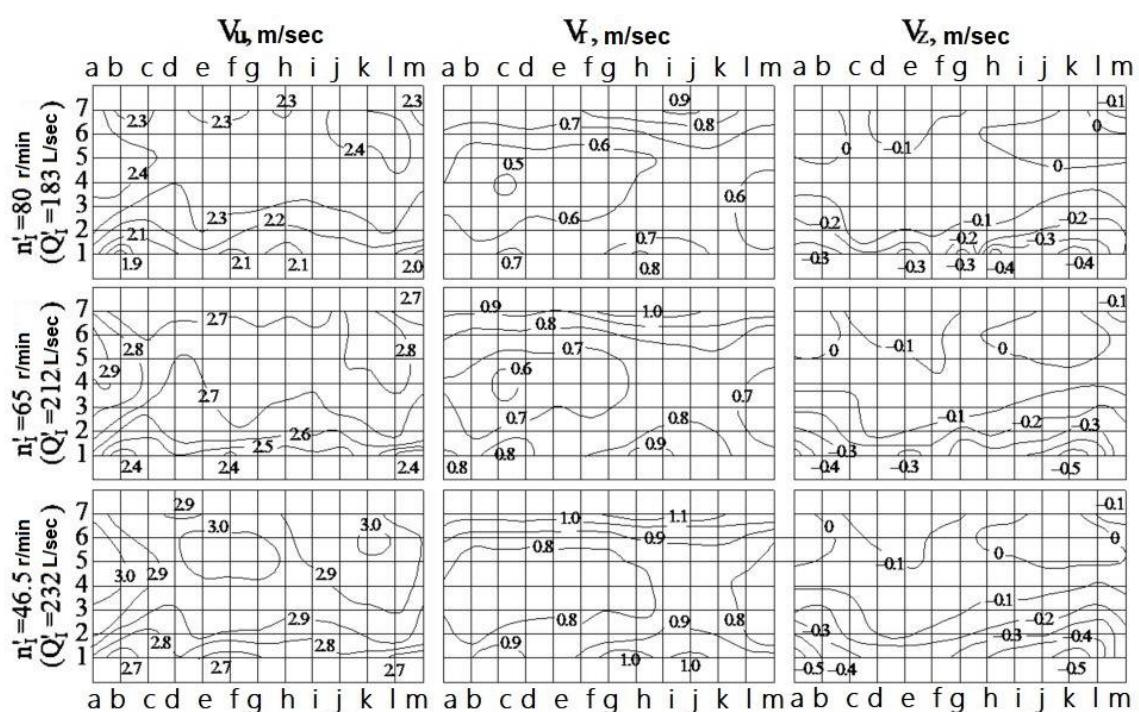
Figure 2. The distribution of flow rates in front of the impeller Francis turbine RO500I-2b ( $D_I = 400 \text{ mm}$ ,  $n'_I = 65 \text{ min}^{-1}$ )
