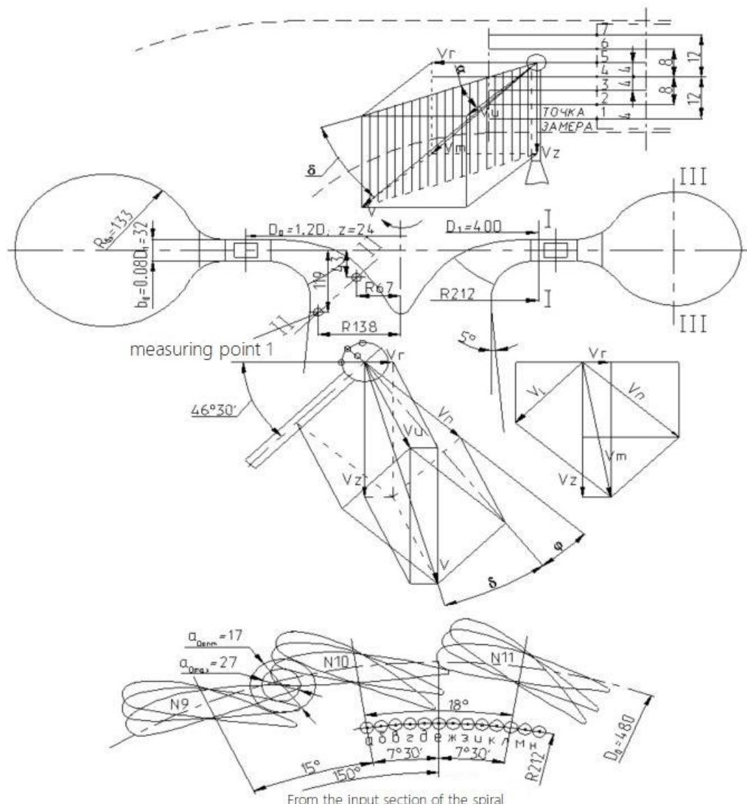
*Figure 1. The location of the dimensional sections in the turbine cavity and the decomposition scheme of the absolute velocity vector*
