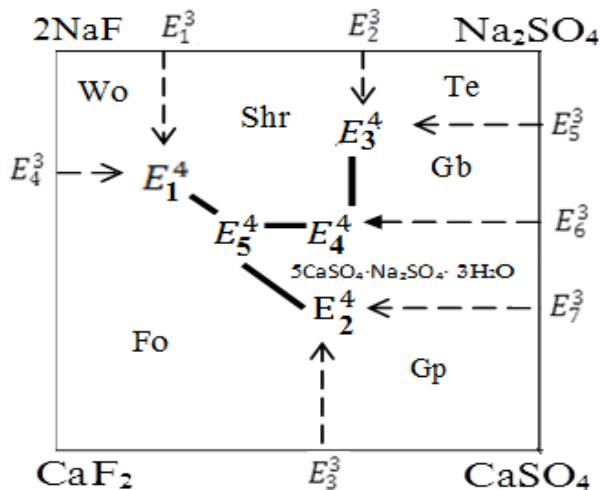
*Fig. 2. Schematic phase equilibria diagram constructed by the translation method for Na, Ca// SO4, F - H<sub>2</sub>O system at 75°C*
