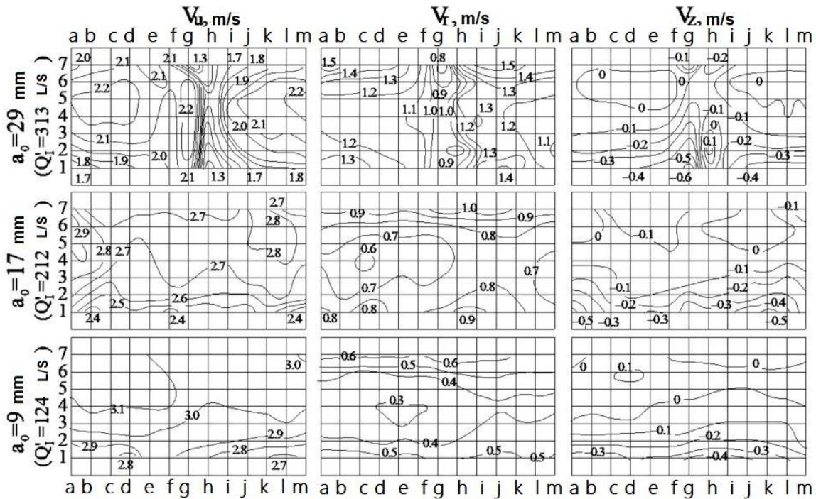
Figure 3. The distribution of flow rates in front of the impeller Francis turbine
