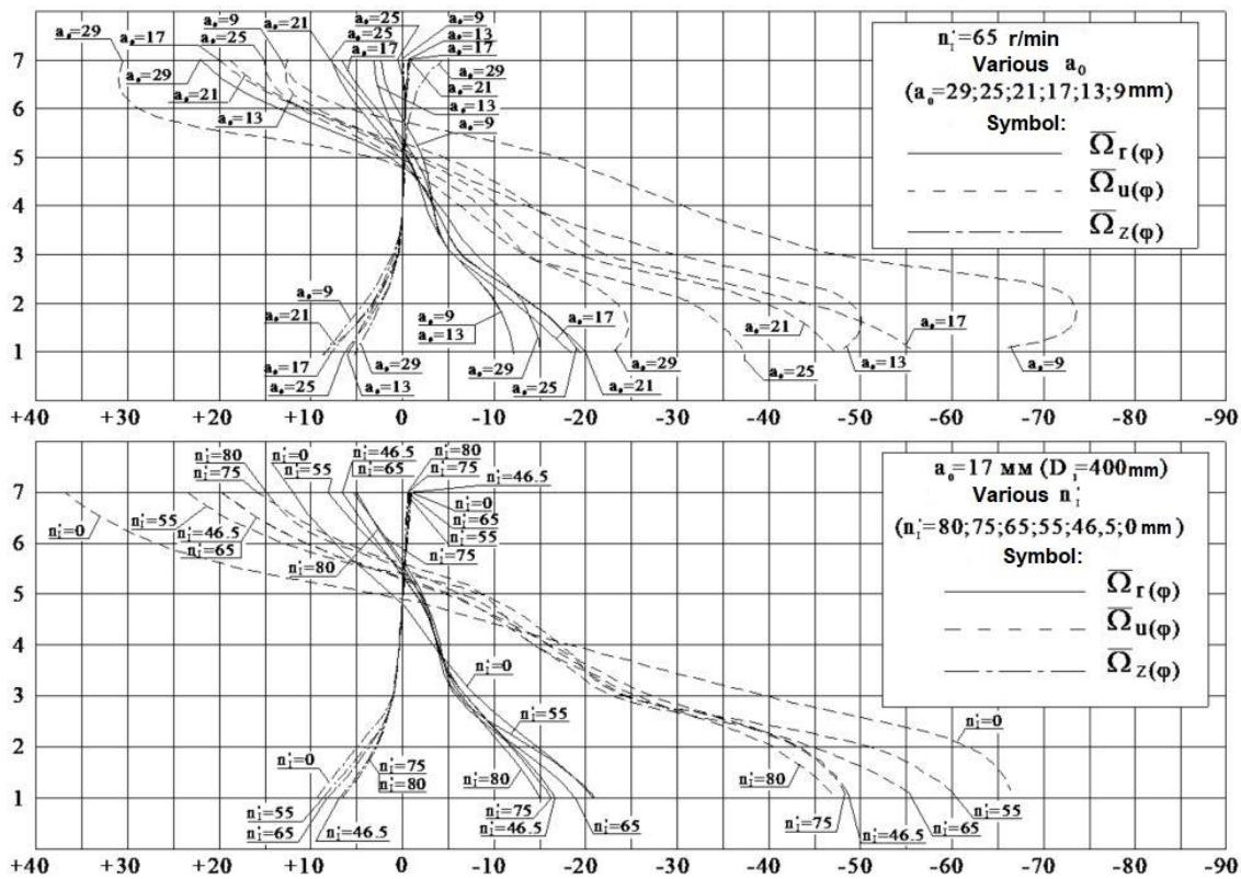
Figure 4. Flow characteristic in section I-I before the impeller Francis turbine
