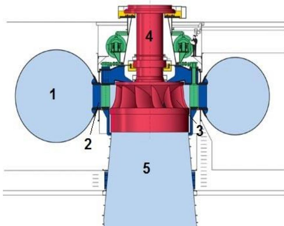
1 – spiral chamber; 2 – guiding vanes; 3 – impeller; 4 – shaft; 5 – draft tube
