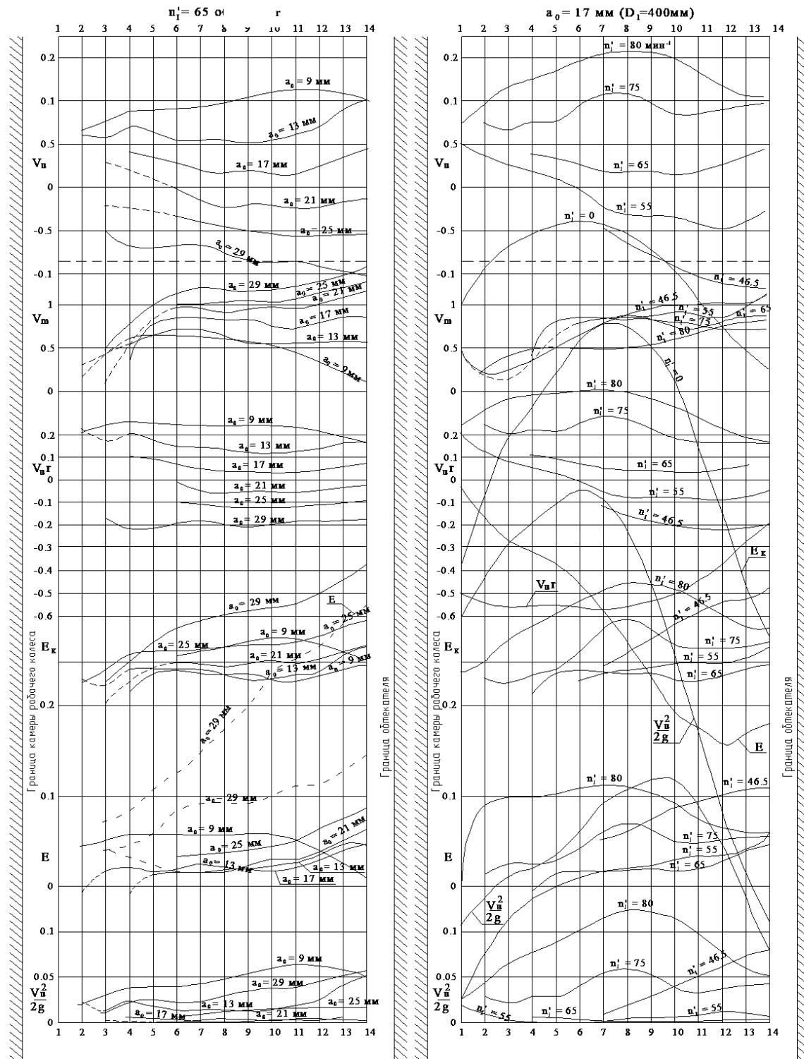
Figure 6. Flow parameters behind the impeller Francis turbine
