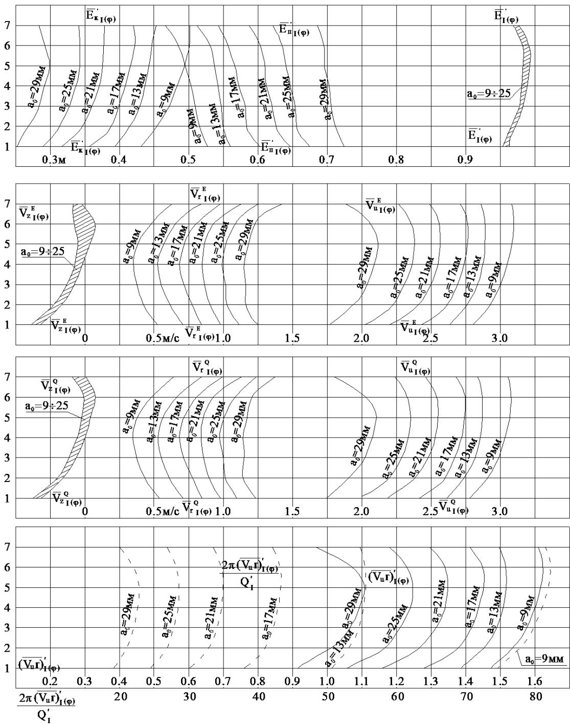
Figure 5. Average flow parameters in front of the impeller Francis turbine
