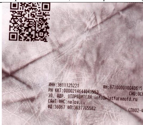
Figure 4. The result of the application of the thermal method of identifying traces of fingers
