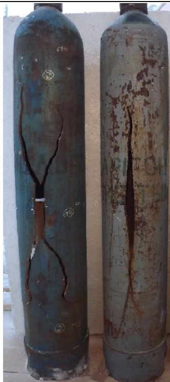
Fig. 8. Vessels after the test. the left one – charged vessel; the right one – vessel with no charge.
